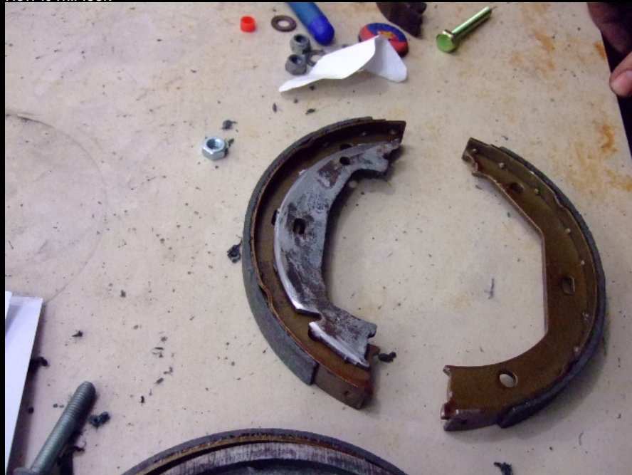
Marking the area to be cut on the 330 shoe
