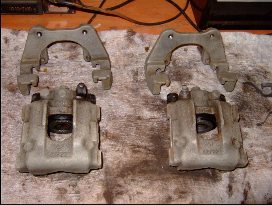
After 2 days in rust inhibitor and more cleaning:
