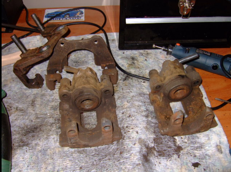
Rear calipers, rusted, ready for their transformation
