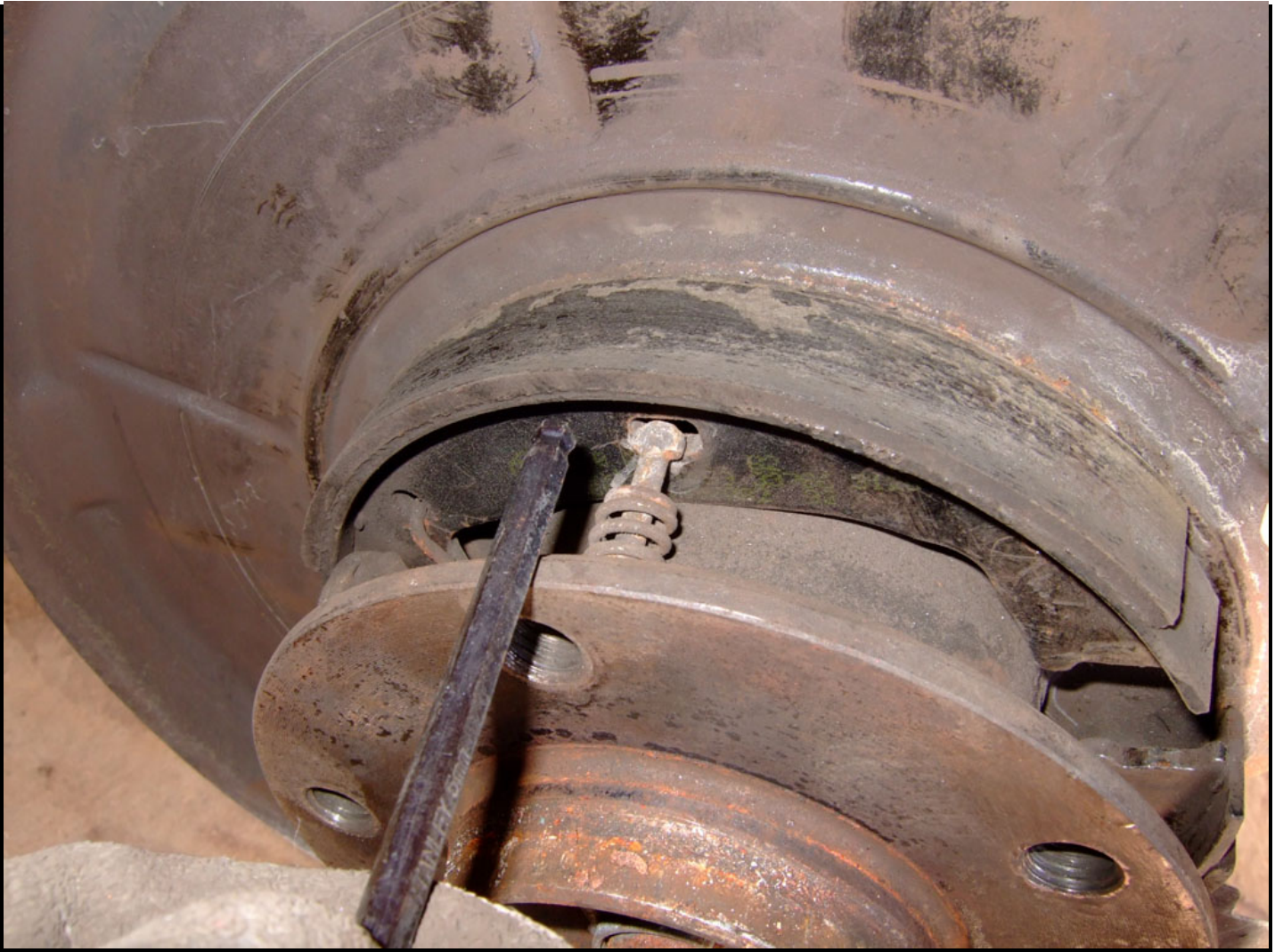
Reassembly using the new hybrid brake shoes to test fit!
