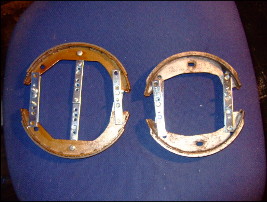
Time to cut the shoes to fabricate the franken-shoe :)
