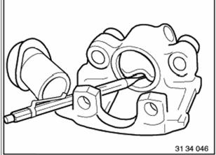
Remove sealing ring carefully with a plastic needle.
