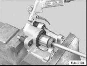
Support brake piston with commercially available extension and socket and press gently onto dust sleeve.
