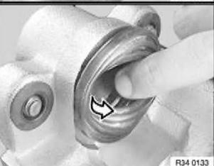
Insert dust sleeve in front annular groove and press into annular groove over entire diameter.
