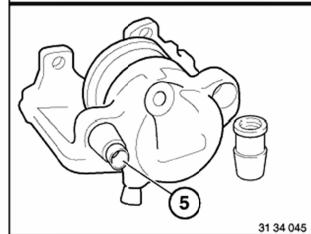
Check guide sleeves (5), fitting repair-kit guide sleeve if necessary.
