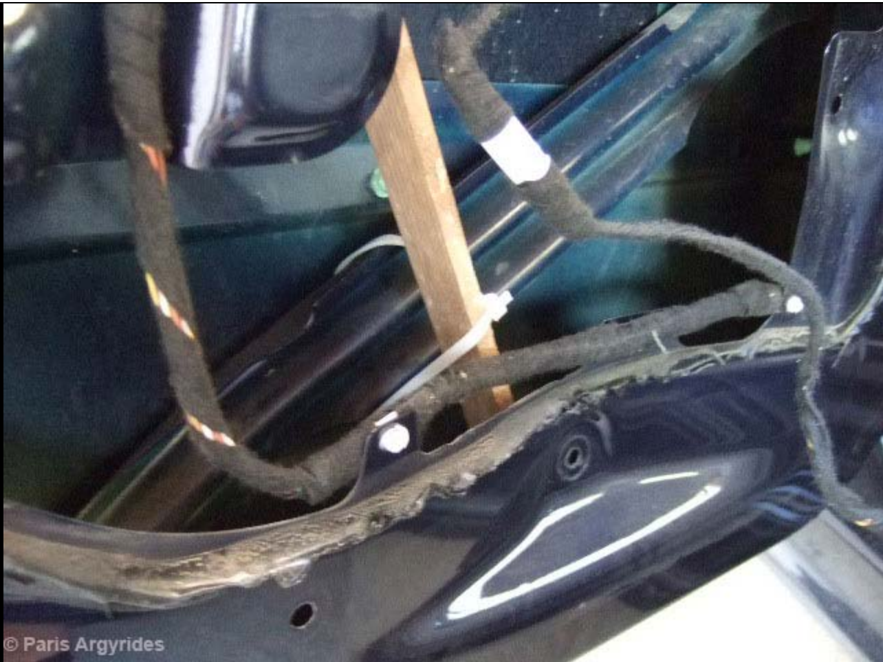
Mechanism in place and secured with the original nuts.
