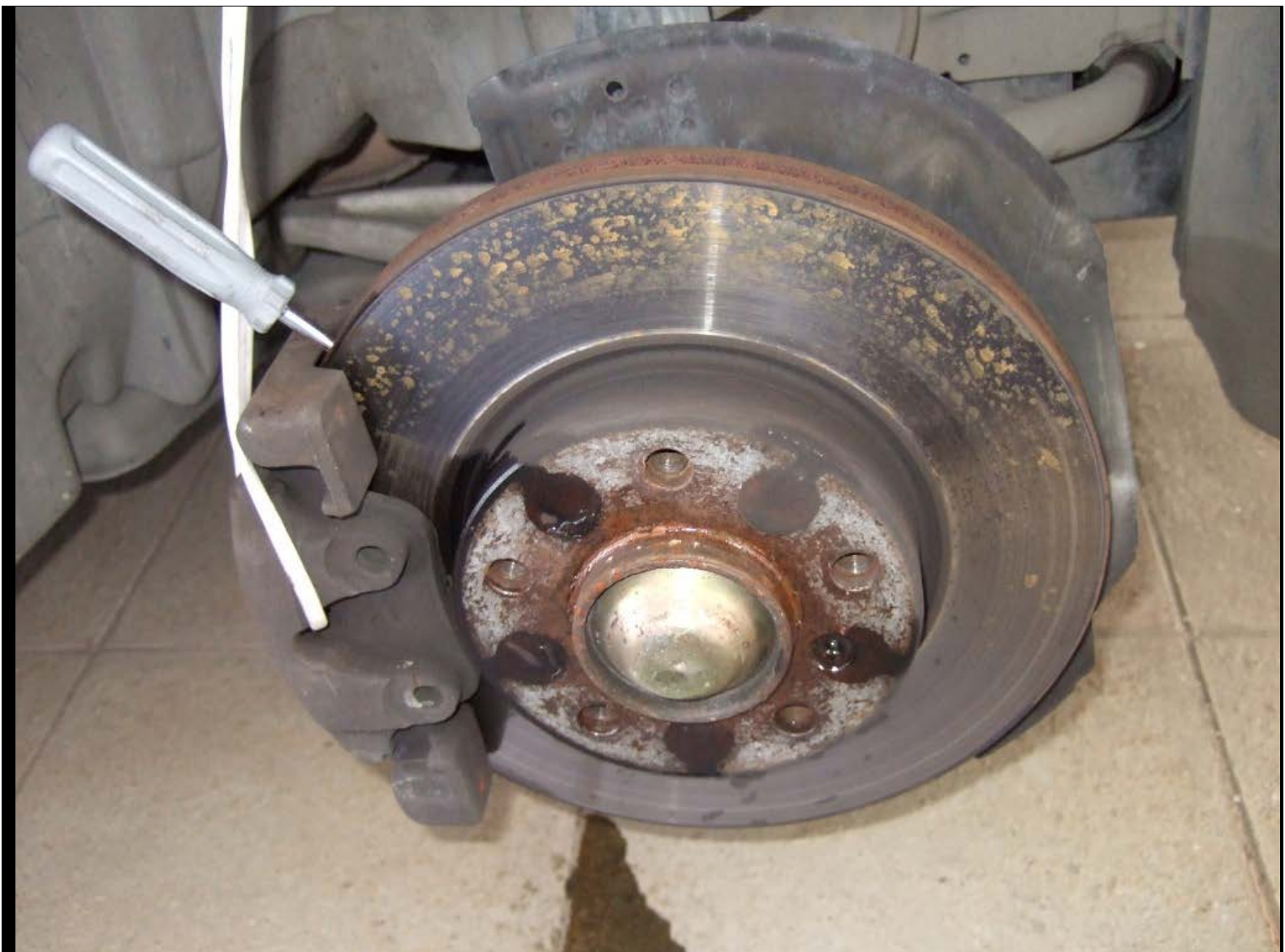
Removed the 2 x 16mm caliper bolts and voila, came out immediately. Everything came out easily, probably because the previous time I torqued them properly. With a bit of hammering, the rotor broke loose too.
