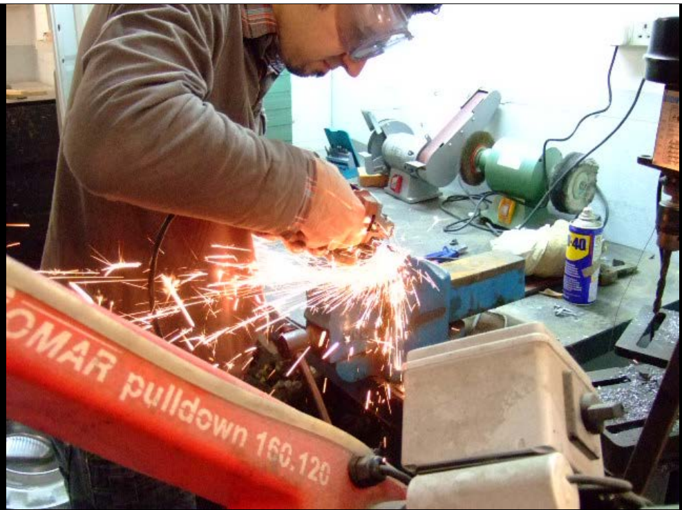
Removing the braking plate out of the 320 shoe
