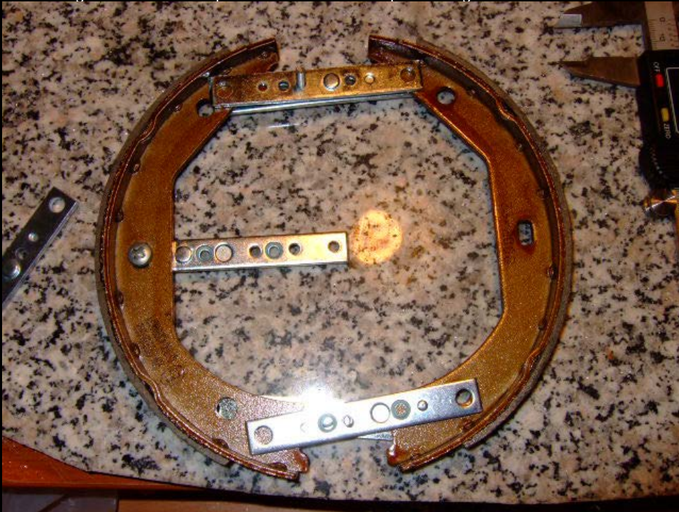
Fabricating some holders to preserve diameter and positioning of shoes so that I don't have to carry the disk with me all the time
