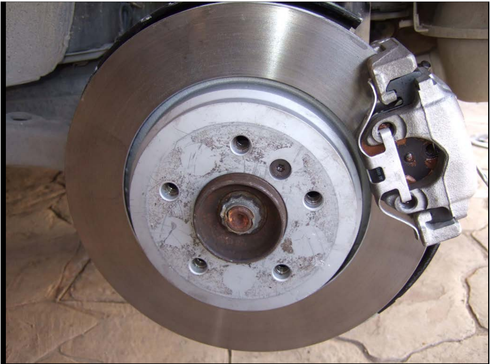
End result with new pads and plates installed.
