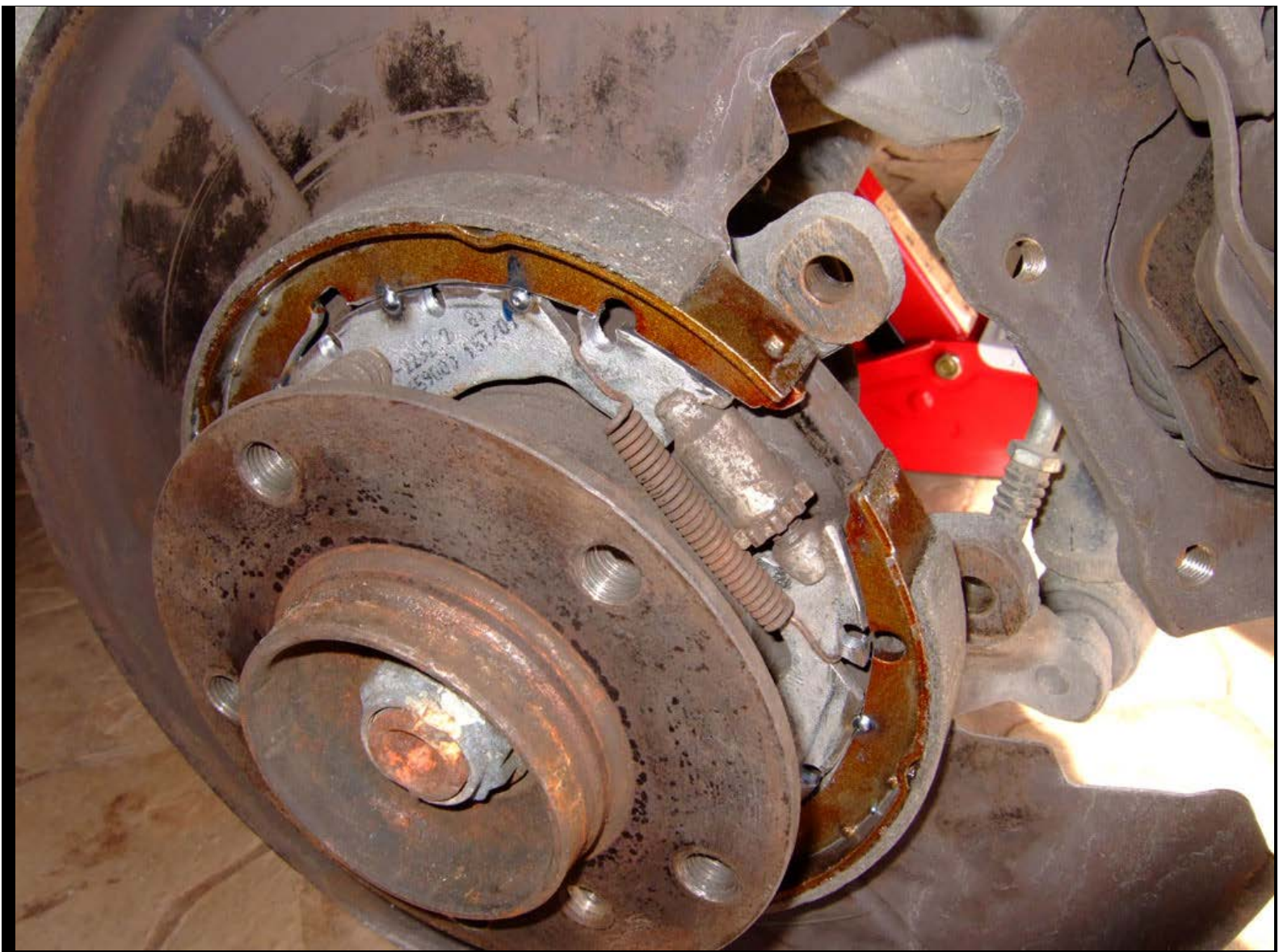
The dust shield took a beating since it was in the way of the larger 330 rotors, I had to bend it out of the way, that is until it's time to do the rear bearings, where I will get a proper 330 based dust shield as well. Unfortunately, without taking the hub apart it's impossible to remove it.
