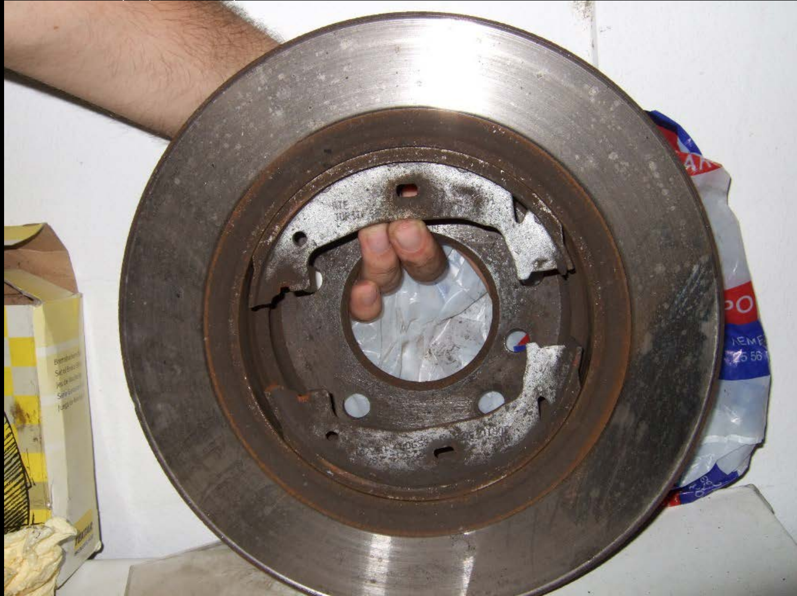
Rear parking shoes below. Manufactured by Meyle. It seems that the shoe part is spot welded on the bracket I want to manufacture. Which
