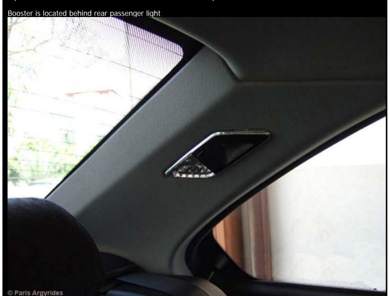
Remove the light by inserting a flat screw driver on one of its sides and prying out. Disconnect the power plug. Behind the light there is a T25 screw that needs to be removed. Then pull the liner until it unclips from the top part. The bottom part is just squeezed in place.
