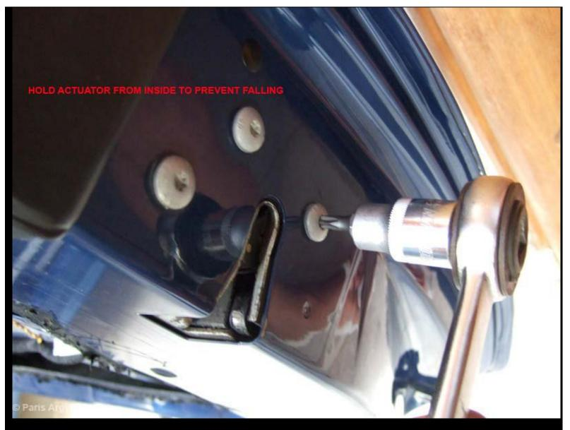
The actuator/lock will fall now and you can remove it from inside the door slowly & carefully by pushing to the left the window rail, to make space. This point I felt that I would break the glass but it managed to survive. You need to push the window guide to the left just as much to allow some space for the actuator to be removed.
