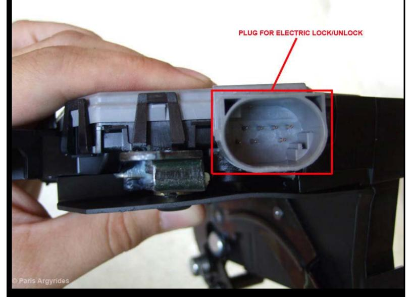
As you can see, all attachments are different so you can't go wrong. For the installation, I chose to connect the door pin shaft only outside the door, then I placed the actuator inside the door, connected the 2 cables (inner + outer handle), screwed it back in place and finally inserted the key lock. After these, I plugged the wire harness back, screwed all the window bolts/nuts.
