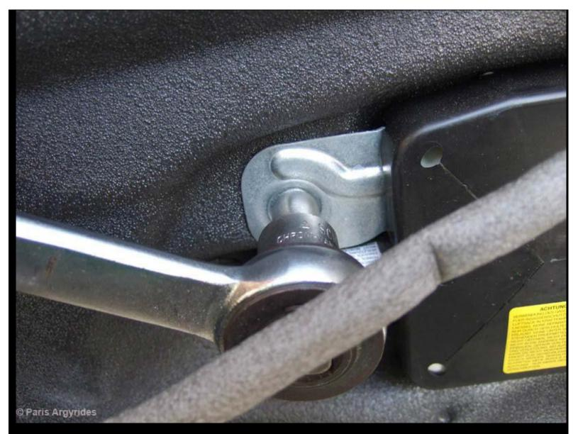
Airbag removed, insulation removed, airbag inserted back.
