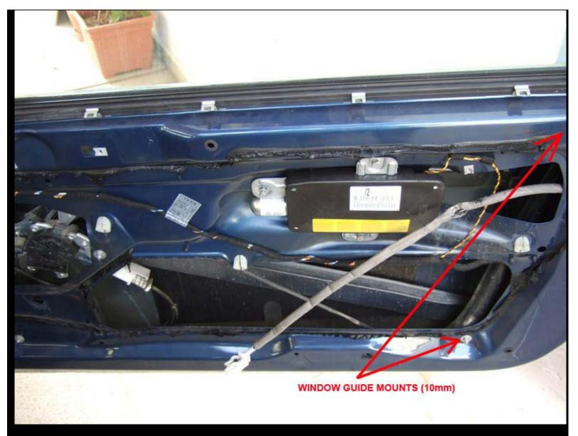
Now it's time to start disconnecting stuff... Twist to release the outer door handle cable as seen below, then slide it out of the holder (yellow part on U shaped metal bracket) Disconnect the wiring harness from the lower right part (not seen in picture) Disconnect the inner door handle as well (not shown too due to lack of space) although you can leave it on until
