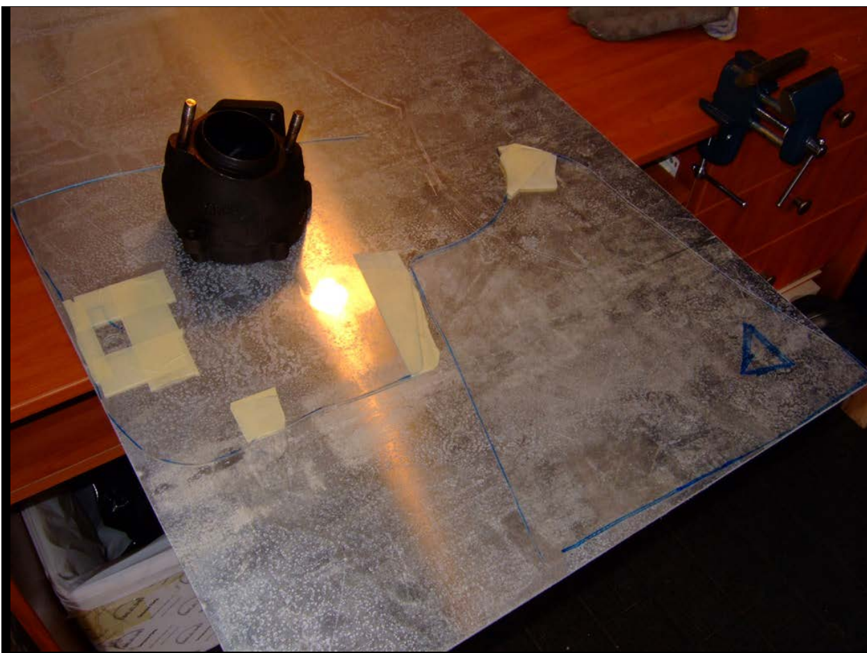
Using a jigsaw and a file, I got it to the proper shape:
