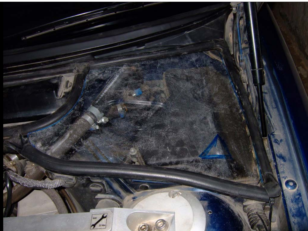
5mm aluminum sheet as the final material for the cover.
