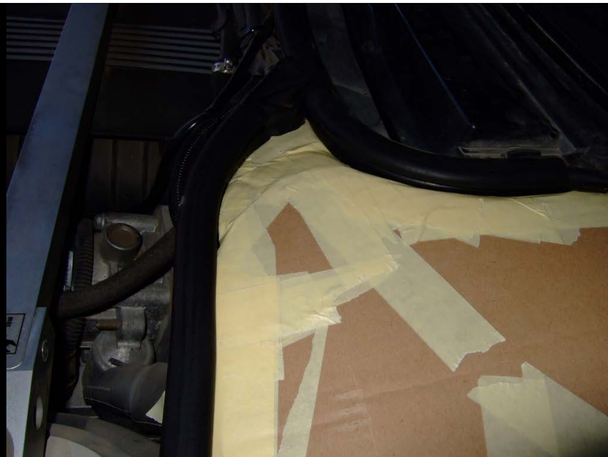
The initial template. I made it a bit larger so that I can shave whatever material I want later on for better fit.
