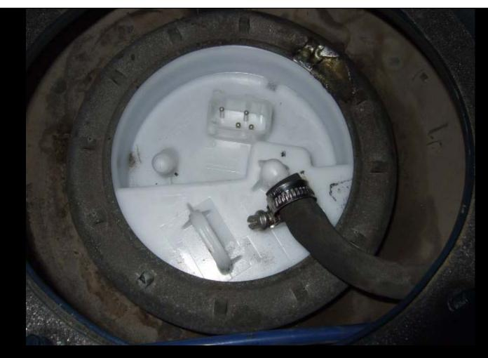
Reconnect the plug, connect the battery and then turn the key to ignition position II, then off, then again on position II so that the pump operates and fills the lines with fuel. Start the car and check for any leaks from the hoses. If everything is ok, re-install everything and enjoy an improved ride.
