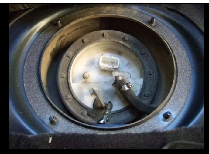
Using a hammer and a screwdriver, lightly hit the big round ring until it becomes loose.
