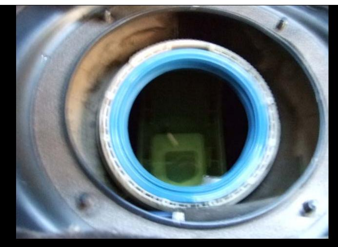
Screw the big metal ring back with light hammer hits, reconnect the fuel hose and secure it with the new clamp
