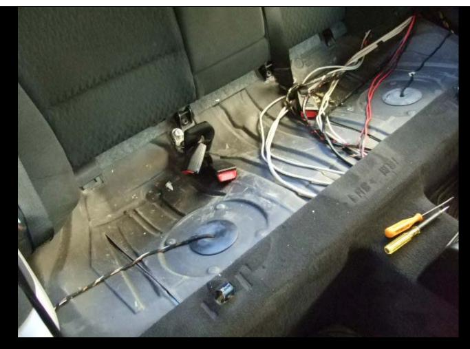
Lift the sound deadening material and undo the 4 nuts that hold the fuel pump access lid
