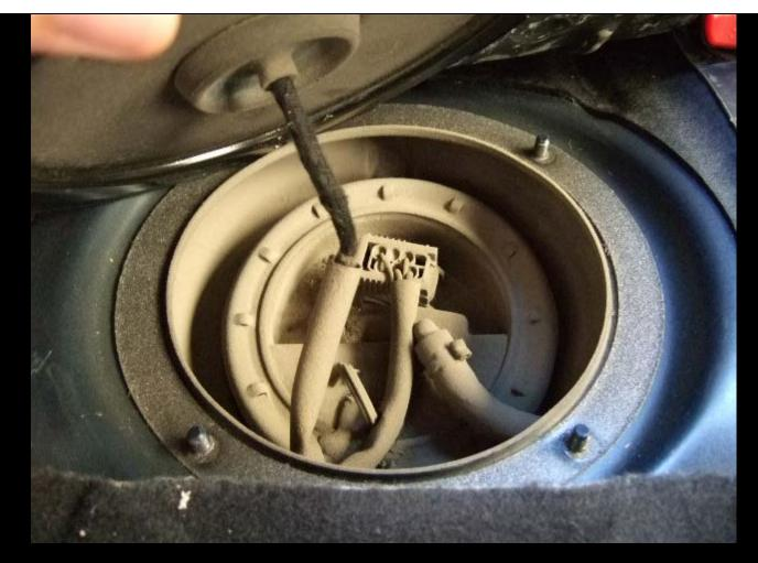
After some vacuuming it looks much better. Disconnect the plug and cut the clip that secures the fuel line on pump. We will be using a new one. Fuel will spill until pressure is relieved so be ready with some rags around. I used a bolt to seal the fuel pump hose to prevent more fuel spilling. Then I used a lot of water to wash out the excessive fuel and cleaned the whole area.
