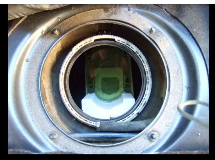
With the new fuel pump and baffle, I also got a new o-ring. Place the o-ring in place before dropping the new pump inside.
