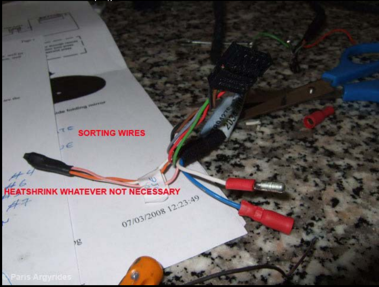
Pressed and soldered plugs on the 2 wires
