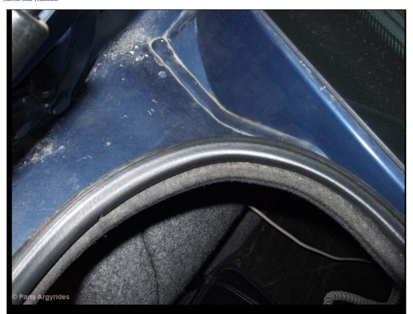
I applied the grease using a rubber glove and wiped the excess. From a first view, the seal looks like new. It's shiny black, softer and will block water better than before.
