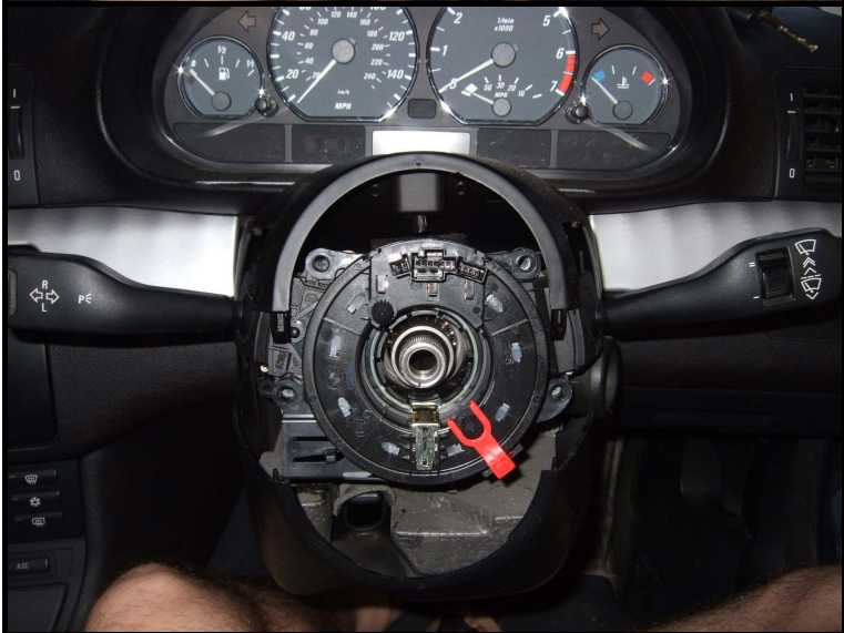
Put the vibration bit and disconnect the indicator, wipers, and steering control plugs.
