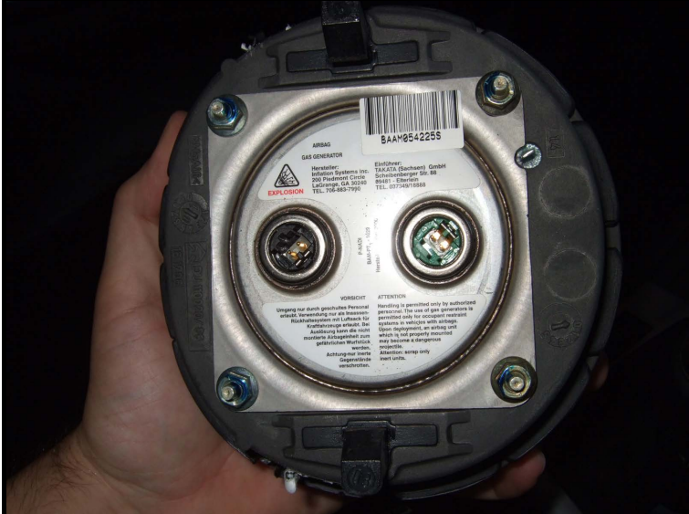
Disconnect the 2 plugs from the wiring. There are locking plugs, so you need to use a flathead screwdriver to pop the lock on each plug in order to pull it out without breaking anything.
