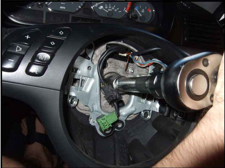
Notes the alignment mark on the steering wheel and on the shaft, this is to be able to place the steering wheel to the correct position.
