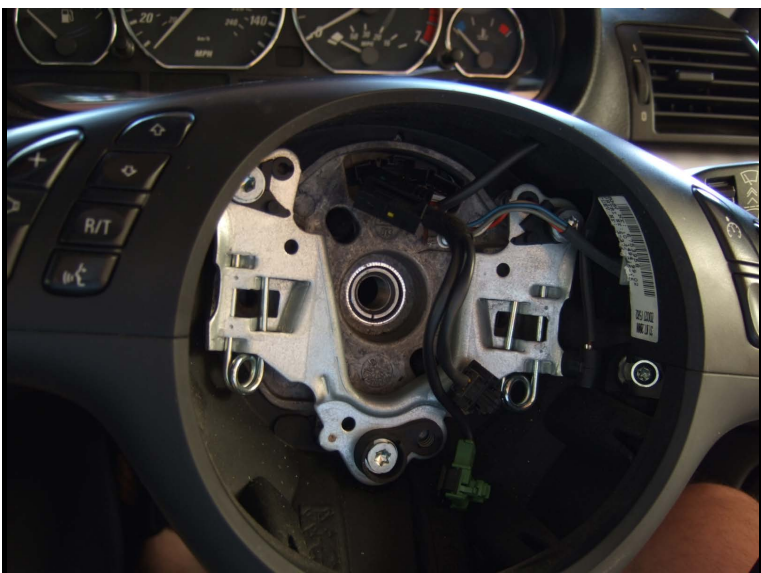
Once the steering wheel is out, you will see the slipring with the wires attached on it. In order to remove it, the upper and lower steering shaft covers must be lifted slightly. There is 1 plastic phillips screw on the top cover and one L-LOCK push/lock pin on the bottom cover. Remove both.
