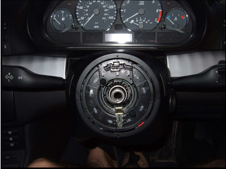
Insert the steering wheel back - align - reposition all plugs - ensure the 1st plug back and fully - plug in the 2nd plug, making sure they are locked on. Put the spring on the steering wheel in position and push it in until it locks in place.
