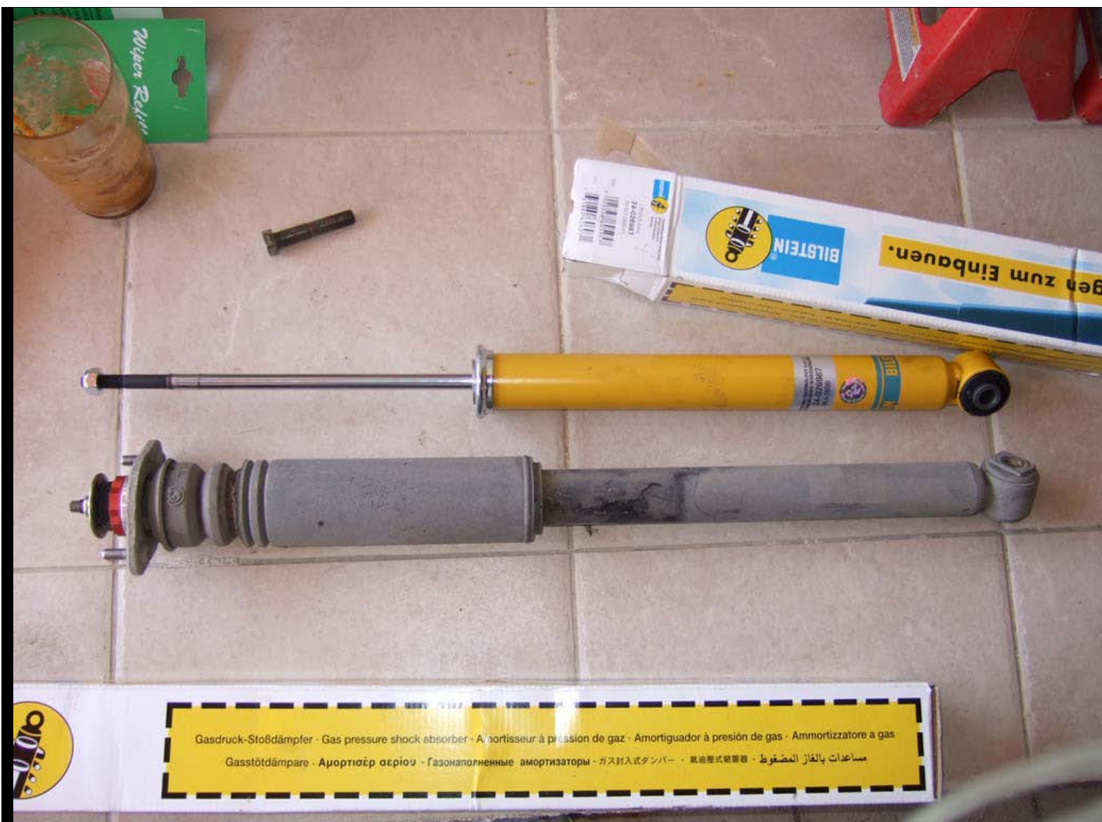
Removed the stock nut on the OEM shock in order to reuse the rear shock mounts, bump stops and covers.
