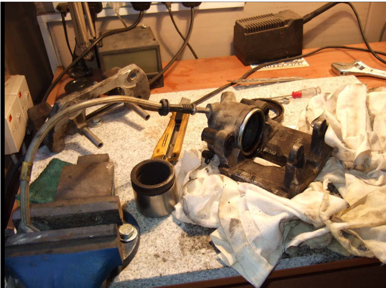
Piston had slight rust that had penetrated just a bit after the cover, but not a big deal. Rest of the piston and bore where perfect.
