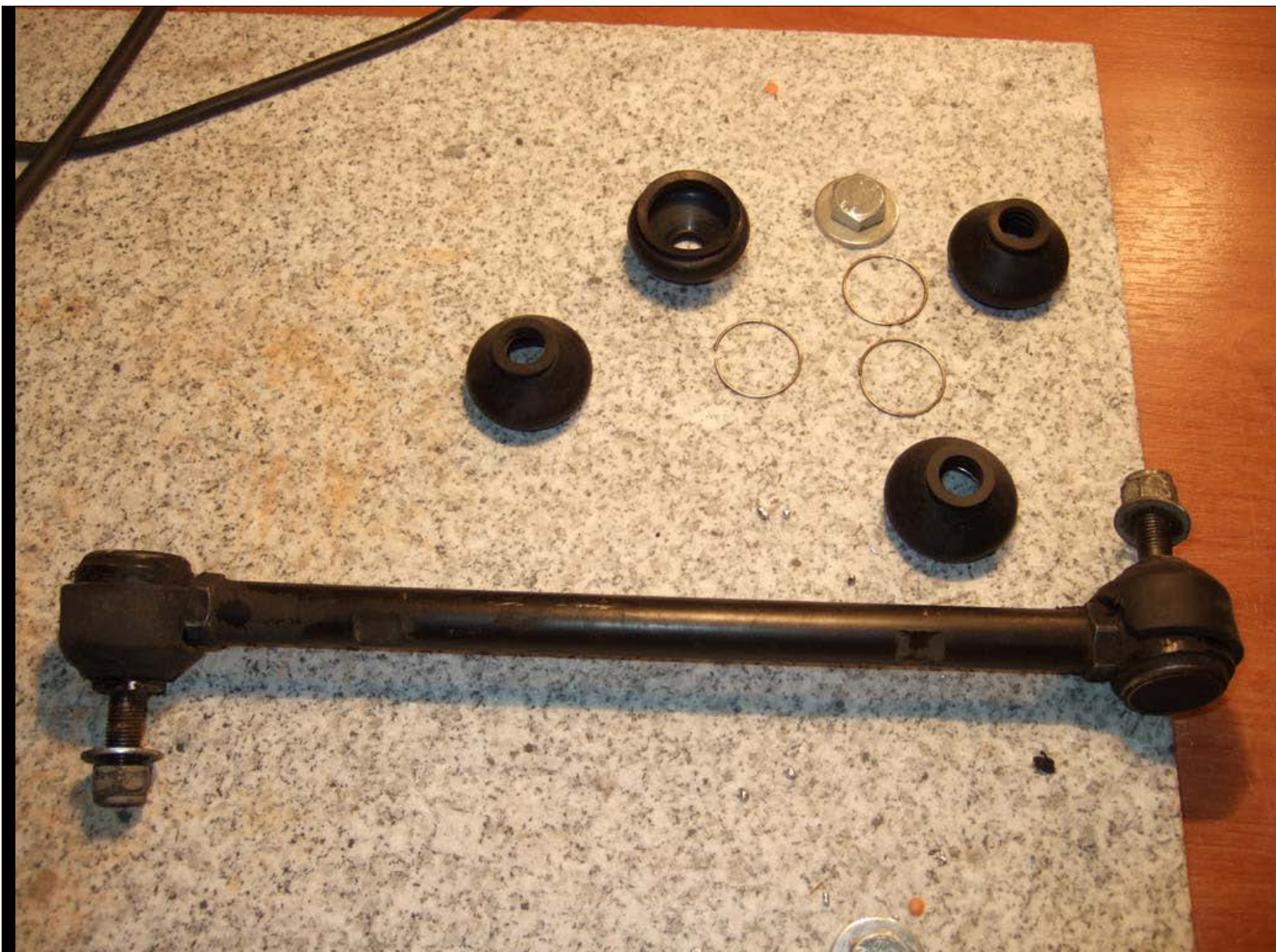
Removed ball joint from rod and thoroughly cleaned
