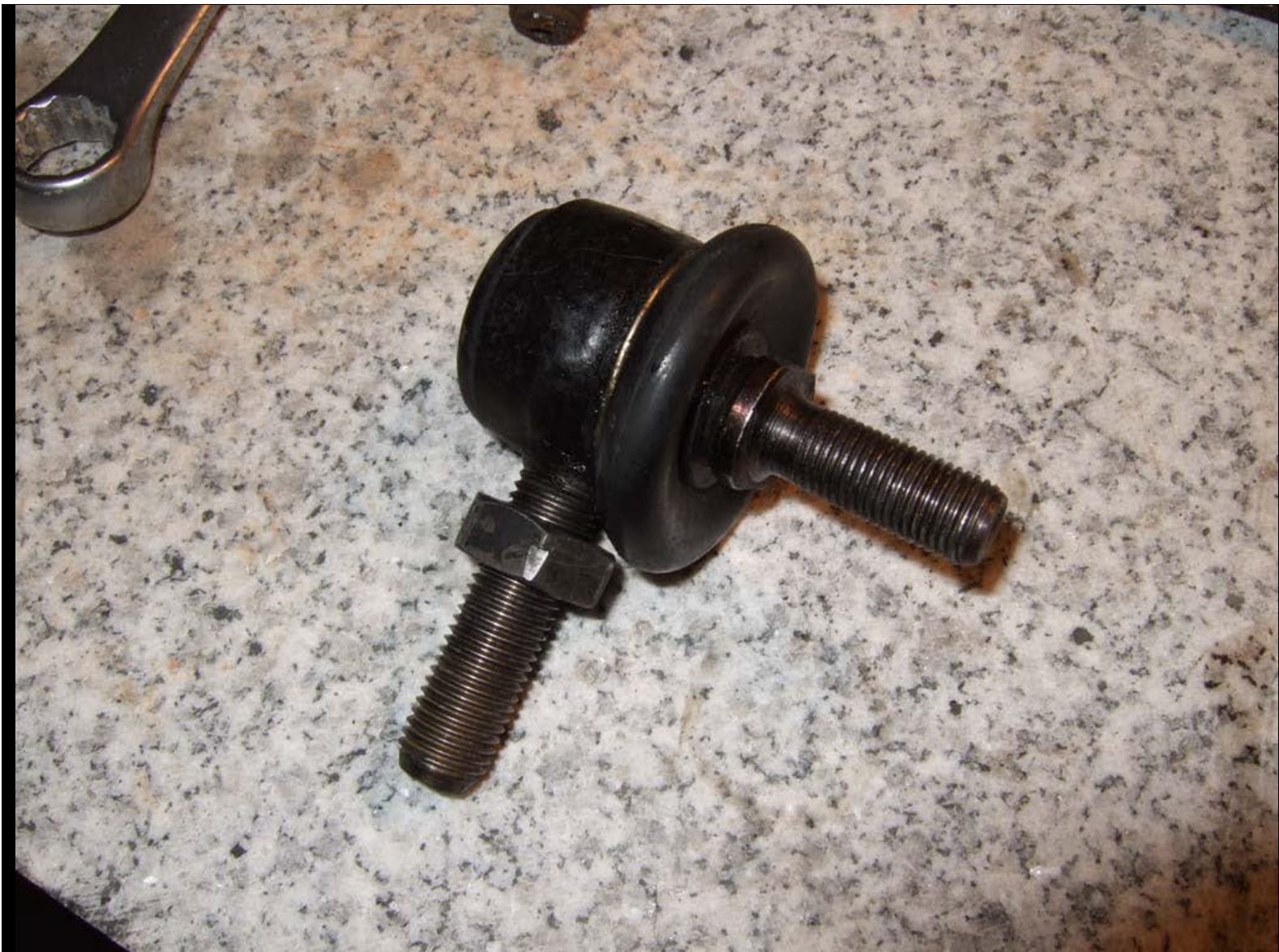
Screwing the ball joints on the endlink rod. I also used locktite so that nothing gets unscrewed accidentally.
