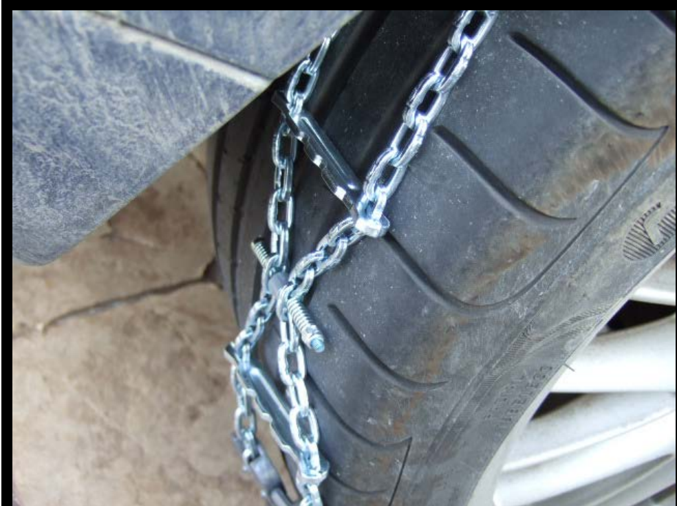
Once the bolt is tight, start ratcheting until the red stitch shows, this means to stop ratcheting.
