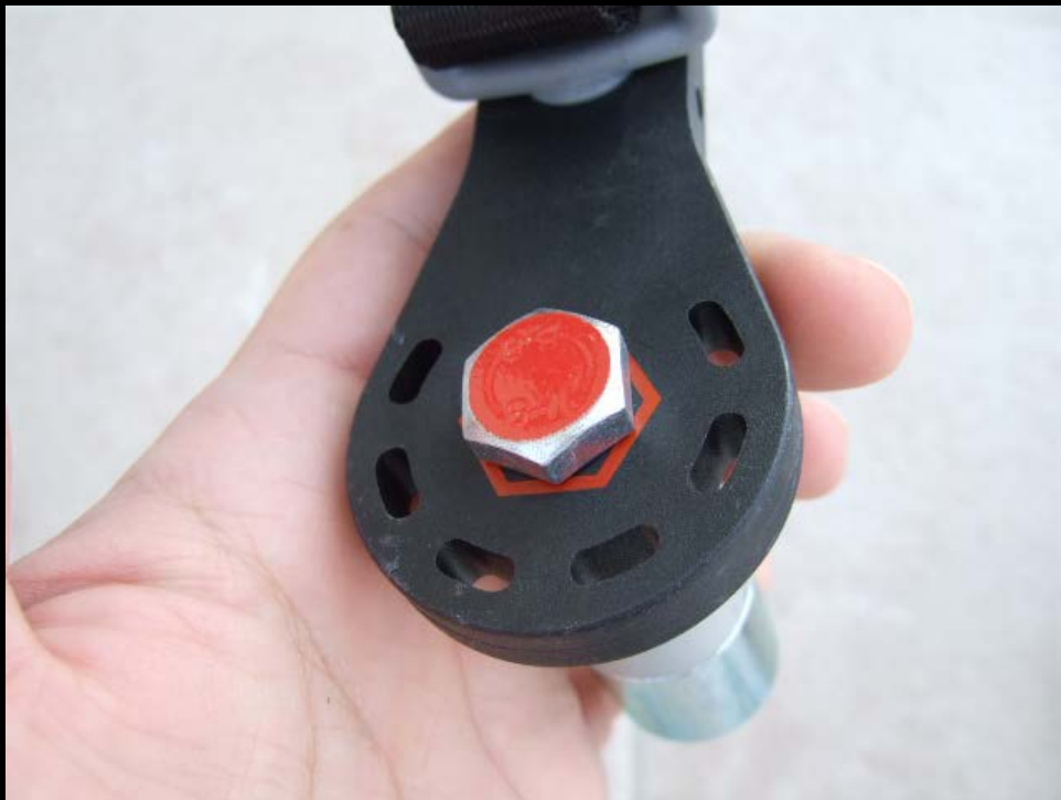
The mechanism that attaches to the wheel bolt
