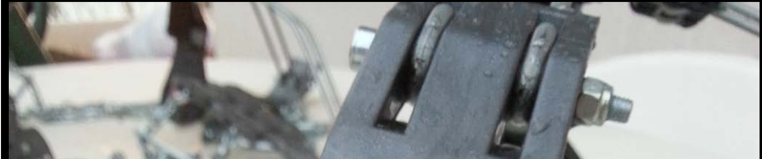
After driving on mixed surfaces, I also checked the composite part of the chains for wear and tear. Thankfully nothing to see, apart from some surface scratches
