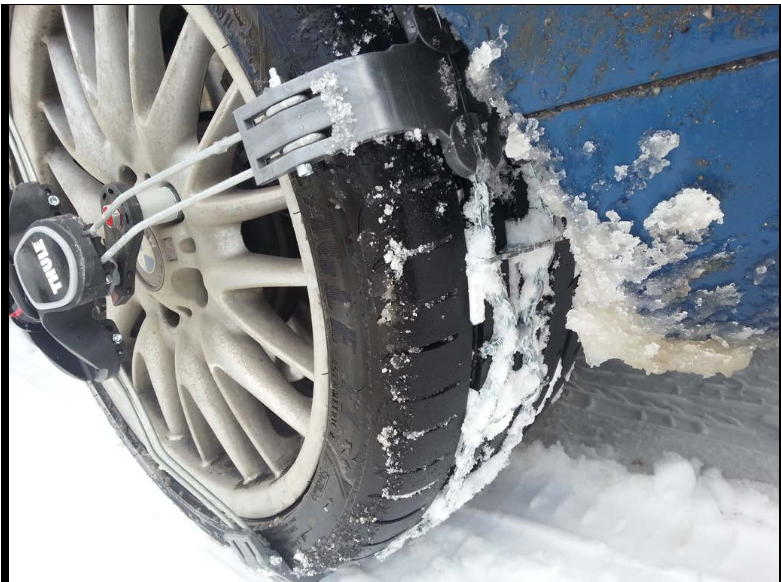
After driving on mixed surfaces, I also checked the composite part of the chains for wear and tear. Thankfully nothing to see, apart from some surface scratches
