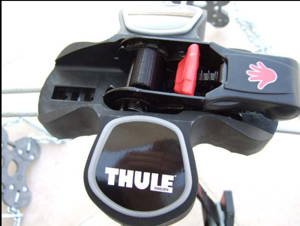
Ratchet mechanism to push the chains on the tire
