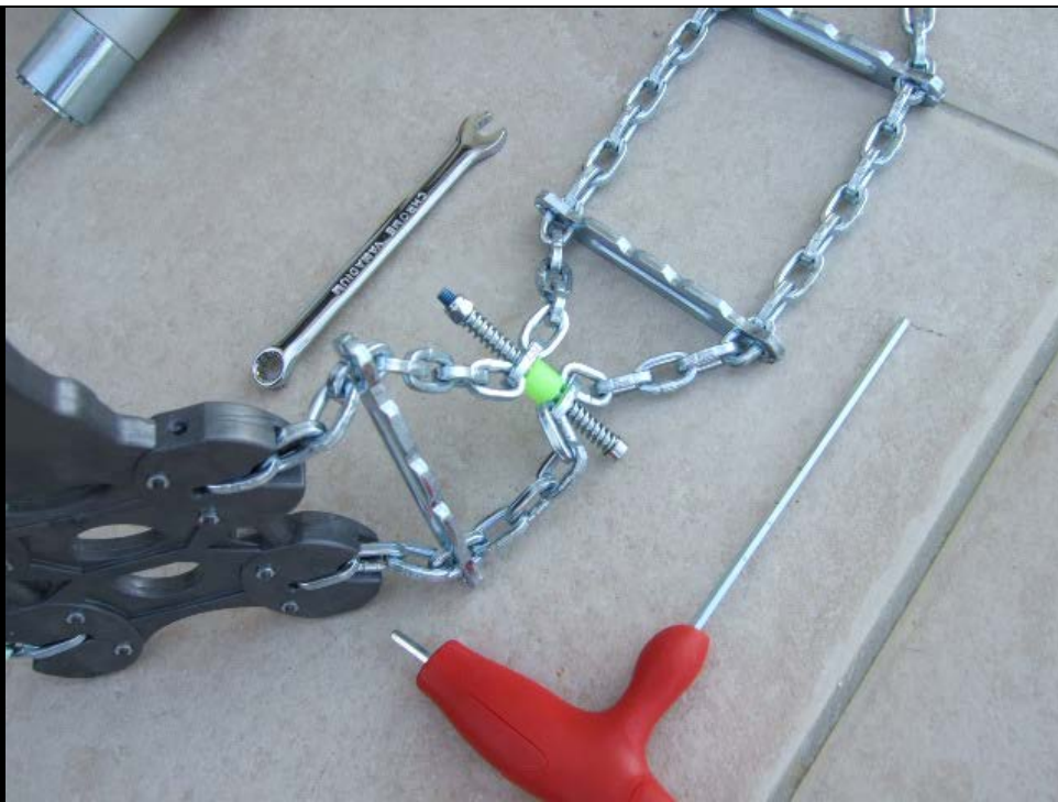
The mechanism that attaches to the wheel bolt
