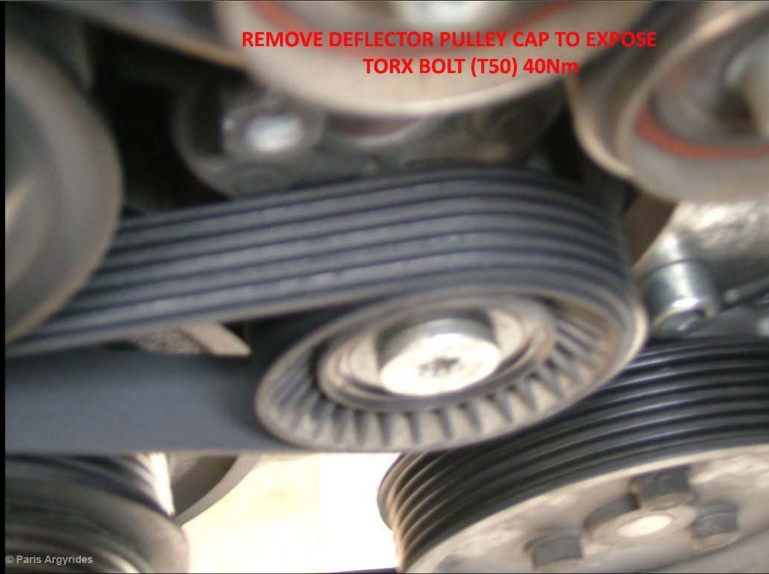
A close-up photograph of an engine's belt system. Several pulleys are visible, with a black serpentine belt wrapped around them. The pulleys have a ribbed design. A red text overlay is positioned at the top center of the image, reading "REMOVE DEFLECTOR PULLEY CAP TO EXPOSE TORX BOLT (T50) 40Nm".
