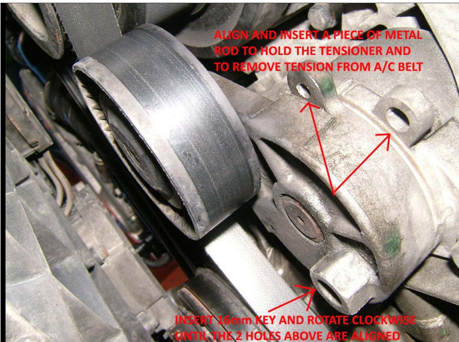
Pop the protection cap from the pulley and insert a T50 bit and remove the bolt. The pulley just drops. Replace it with new one and tight back to 35-40Nm. Re-install protection cap and you are done!
