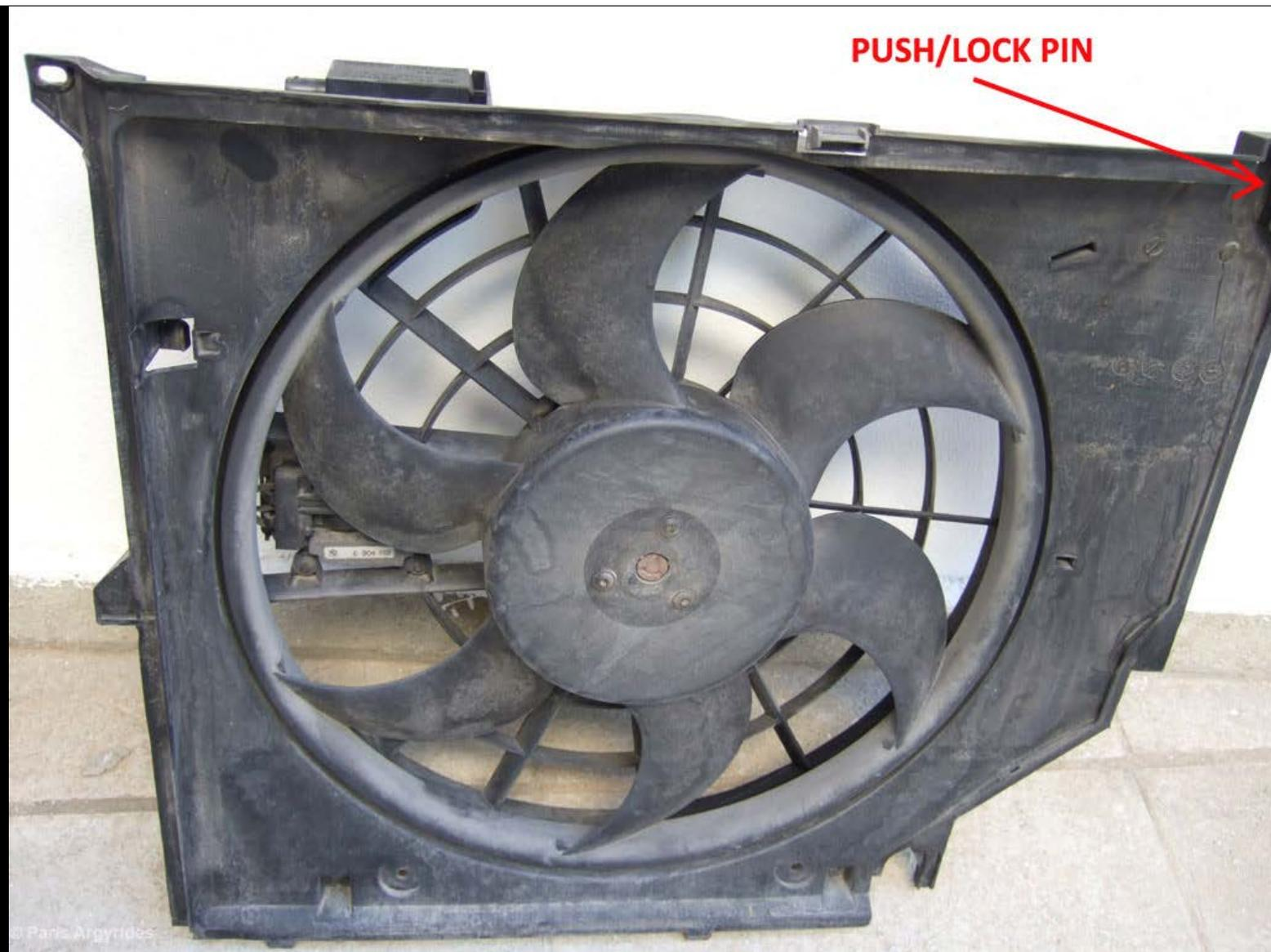
Remove both plugs and the T25 torx screw on the left. Lift it and it's out of the way. 5 Minutes!!
