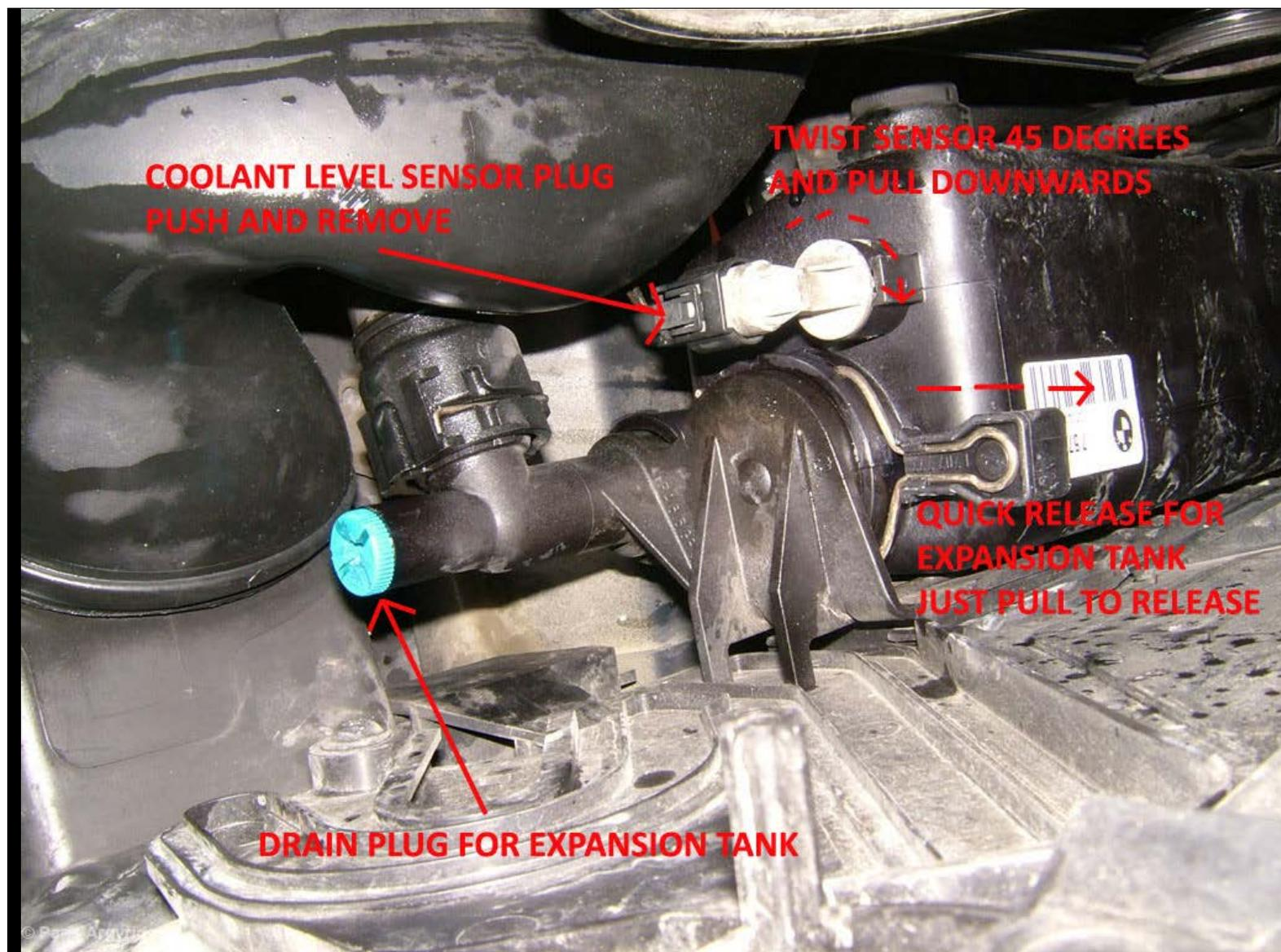
Remove plastic bleed screw, radiator cap and 2 quick release springs from upper radiator hose.
