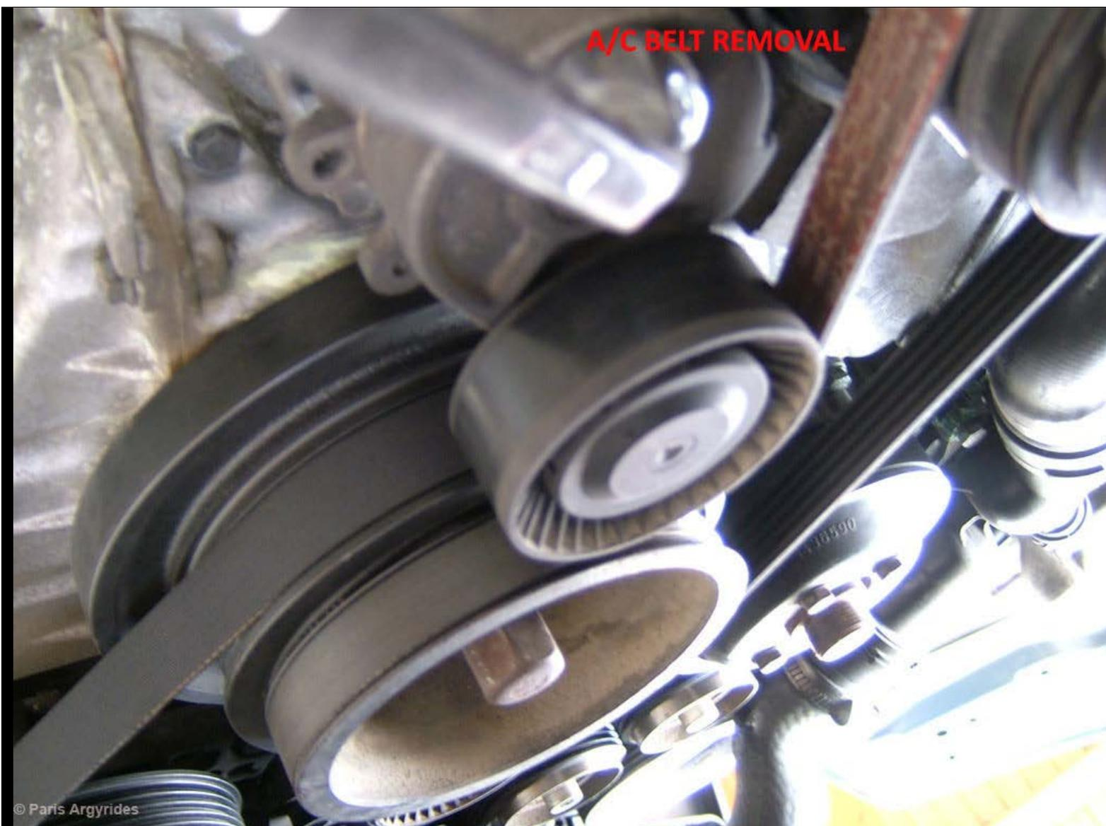
When the 2 holes shown below are aligned, insert a metal rod like an allen key to hold the spring compressed. Now remove the A/C belt
