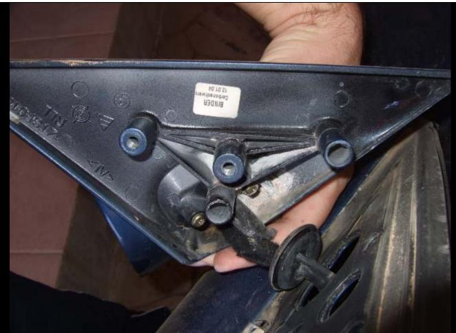
Once tight, replace the foamy gasket, grab the rubber grommet from the inside and pull it until it goes back in to place. <- Important step else water might enter the door card and you don't want this to happen! Re-install the 2x10mm bolts and finally re-insert the black cover. The plastic cover first goes in the bottom hole, then you push it downwards and then you push the top section to clip in place. It's pretty intuitive.
