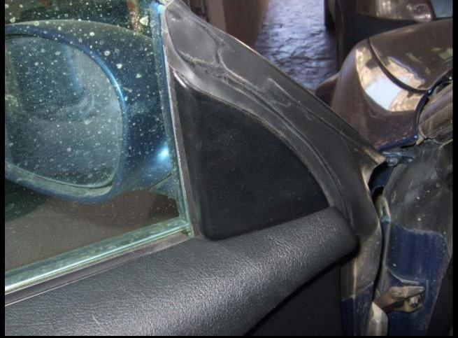
See the bottom hole how it is shaped, that's why you need to pull upwards when the top part unclips. Now remove the 2x 10mm bolts while holding the mirror in place.
